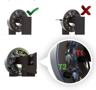
Correct sensor positions for heating with double temperature measurement and ∆T monitoring.
