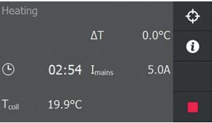
During heating, the pre-set time counts down to 00:00. When 00:00 is reached, the induction heater switches off. The workpiece is then demagnetized automatically and a loud, continuous beep sounds. Press STOP to switch off the beep.
