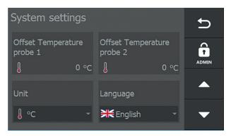
Offset Temperature probe 1: Calibration / correction readout thermocouple 1
