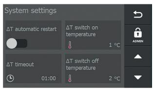
The temperatures T1 and T2 are measured during the heating process. The difference between these two temperatures is calculated continuously. If the difference is larger than the temperature set under " $\Delta T$  switch off", the heating process switches off or pauses.
