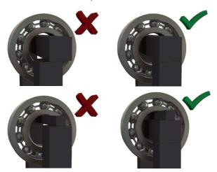
Swivel arm models: swivel the ledge open (towards you) until it drops in the safety positioning cam. Slide the workpiece over the ledge until it is in the middle. Swivel the ledge back to the pole.
