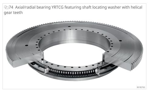
Axial/radial bearings YRTCG are based on the YRTC bearing design. This proven rotary axis bearing solution is available in bore diameters 150 mm to 580 mm as a new variant featuring a shaft washer with helical gear teeth.
