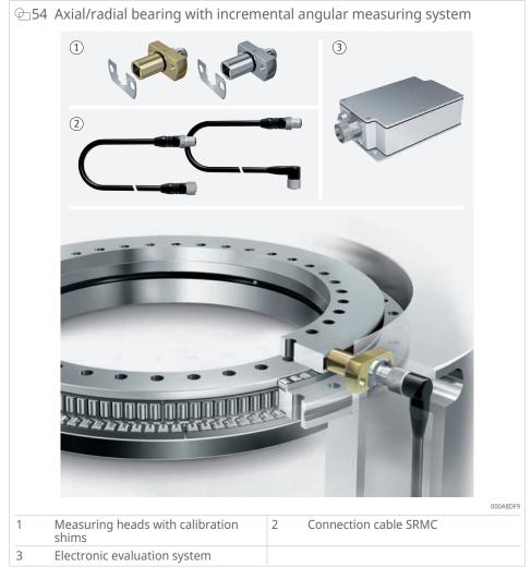
The electronic measuring system SRM comprises two measuring heads, two stacks of calibration shims and an electronic evaluation system. The signal leads SRMC for connecting the measuring heads to the electronic evaluation system can be ordered individually in various designs.
